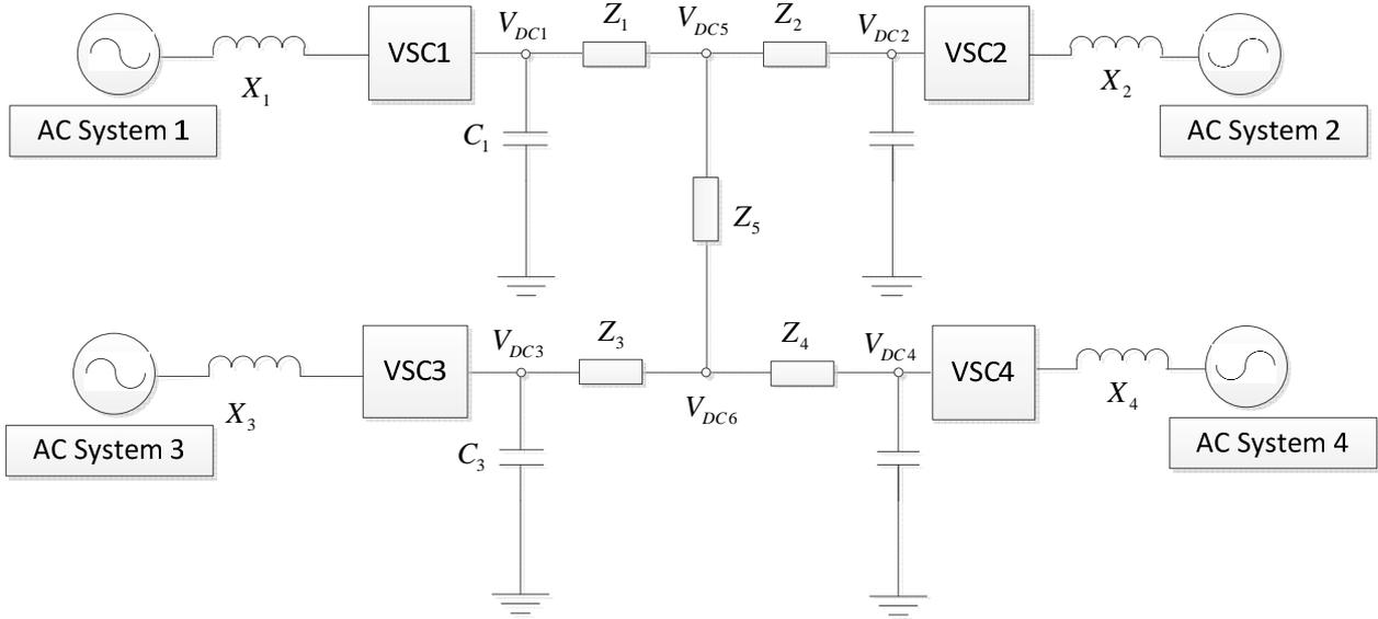
**Figure 6 - Example of a radially-connected VSC-HVDC MTDC network with four terminals.**
