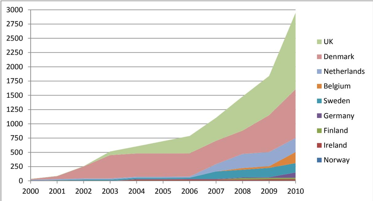
**Figure 1 – Offshore wind energy accumulated installed capacity in Europe in the last decade [4].**
