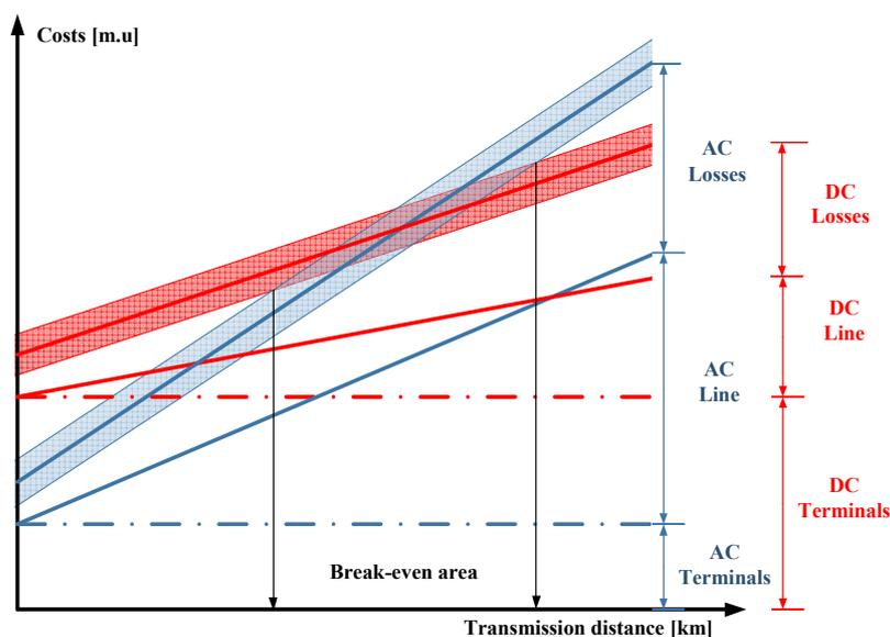
Figure 2 – Cost Comparison between HVAC and HVDC transmission systems.
