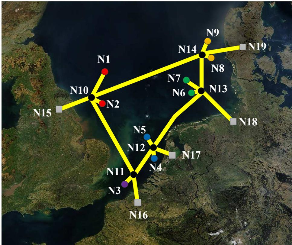
**Figure 7 - NTSG layout for load flow study with five EU countries.**
