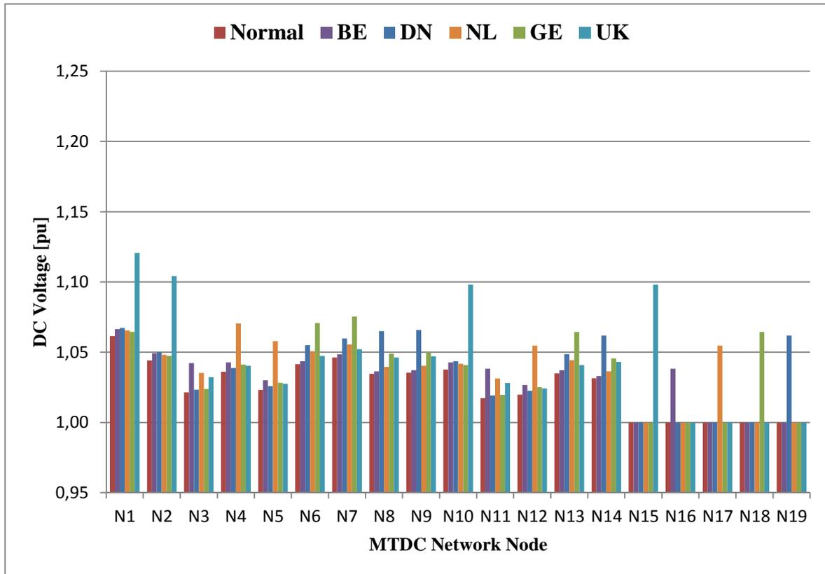
**Figure 10 – Voltage profiles with all 5 countries as slack nodes.**
