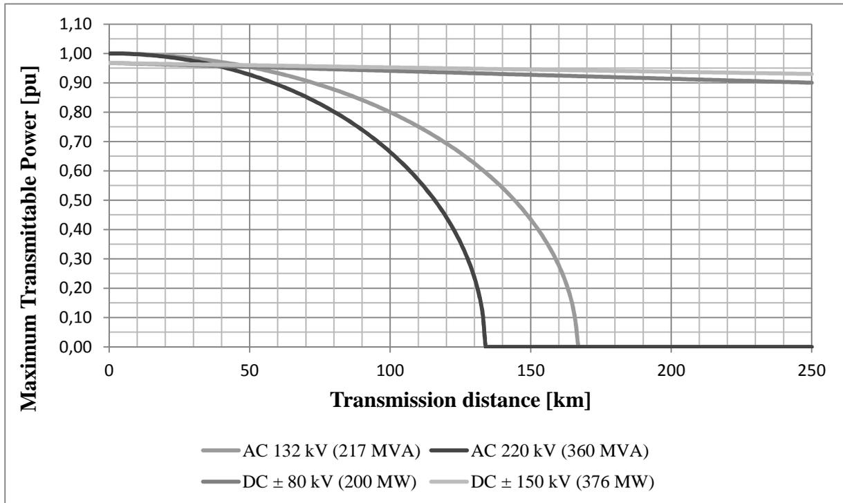
**Figure 3 - Maximum transferrable power as a function of transmission distance for AC and DC submarine cables.**
