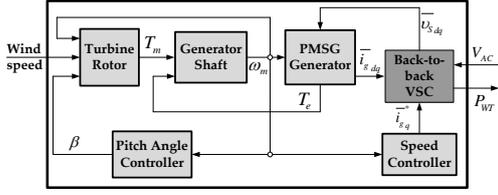
Figure 10: Modular representation of variable-speed PMSG wind turbines.
