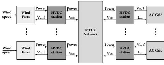
Figure 2: Modular representation of offshore MTDC networks.
