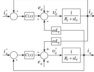
Figure 7: Block diagram representation of the VSC-HVDC state-space equations with feedback control.
