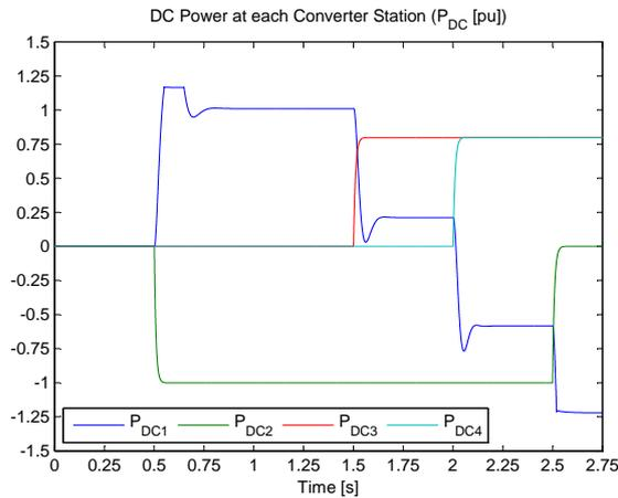
Figure 12: Active power inside the MTDC network.
