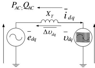
Figure 6: VSC-HVDC station single-phase equivalent circuit.
