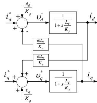
Figure 8: Equivalent block diagram representation of the VSC-HVDC with inner current controller.
