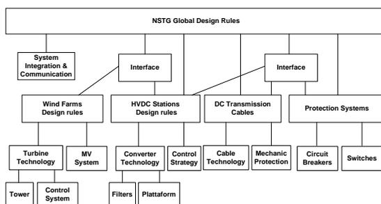
Figure 1: A possible design hierarchy for the NSTG system with four modules.
