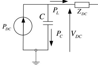
Figure 9: Equivalent circuit of the VSC-HVDC station DC side.
