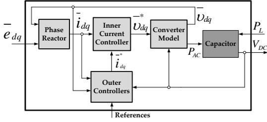
Figure 5: Modular representation of the VSC-HVDC transmission station.
